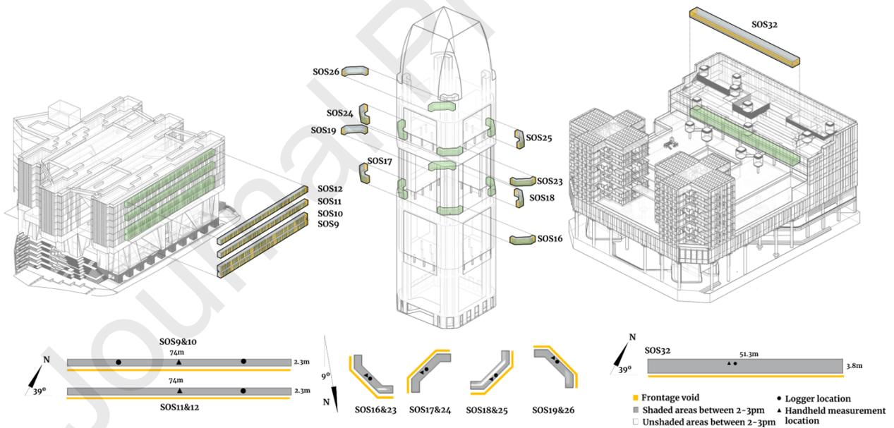
Figure 3. Above: semi-outdoor spaces (SOS) labelled previously as *perimeter buffers*, where yellow colour indicates voids. Below: dimensions, measurement locations and shading conditions between 2 and 3pm (Reference days: SO: June 10; OA: June 26; & KA: July 09).
