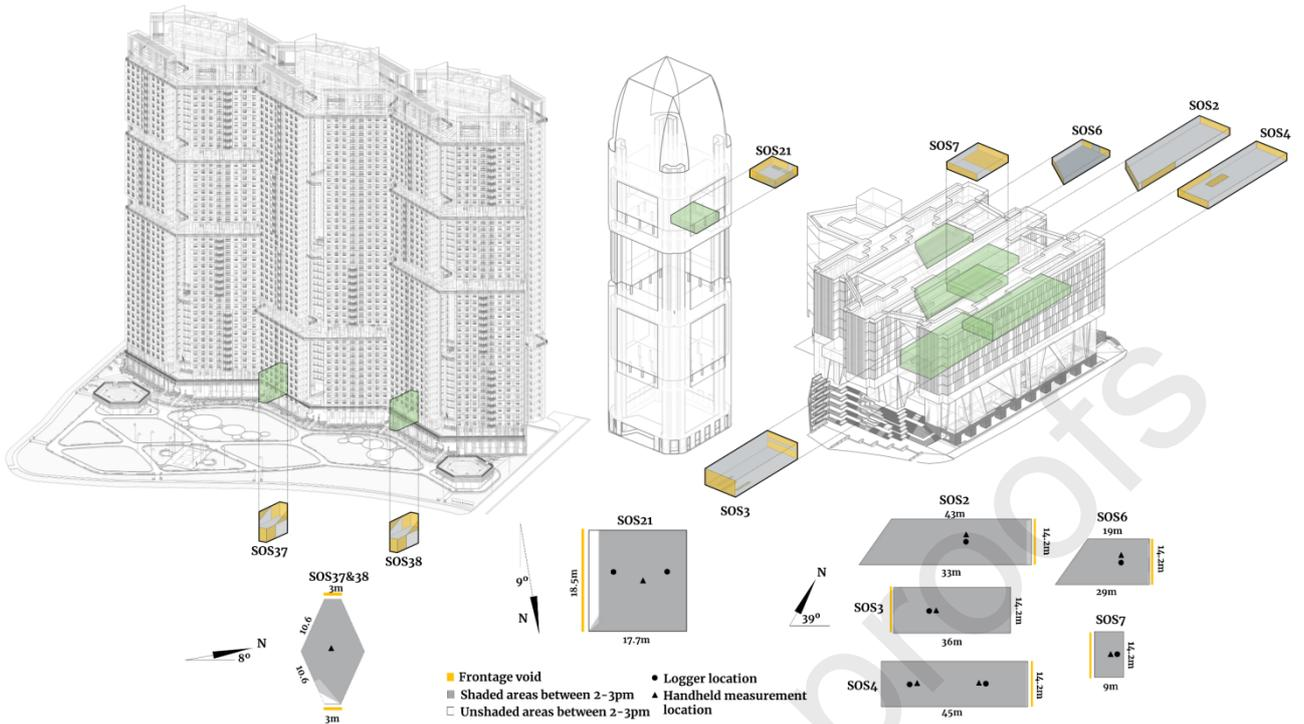
Figure 6. Above: semi-outdoor spaces (SOS) labelled previously as *horizontal breezeways*, where yellow colour indicates voids. Below: dimensions, measurement locations and shading conditions between 2 and 3pm (Reference days: SV: July 24; OA: June 26; & SO: June 10).
