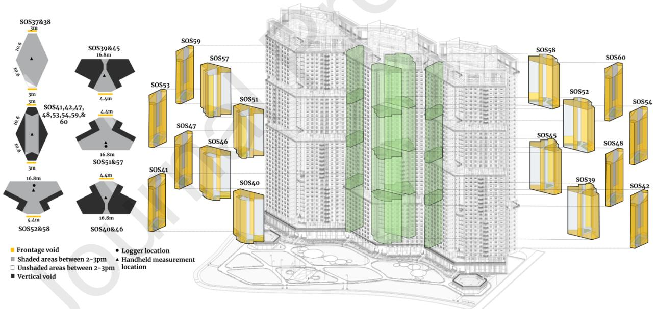
Figure 7. Right: semi-outdoor spaces (SOS) labelled previously as *vertical breezeways*, where yellow colour indicates voids. Left: dimensions, measurement locations and shading conditions between 2 and 3pm (Reference day: SV: July 24).
