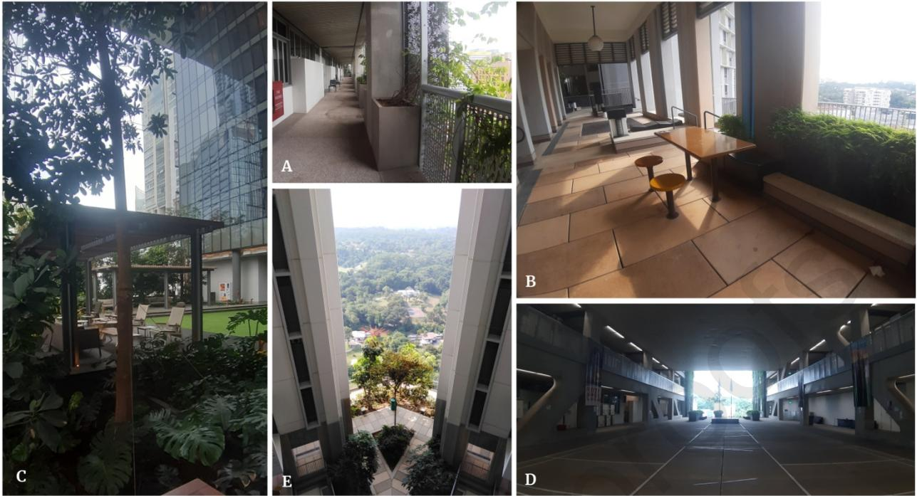
Figure 2. Semi-outdoor space labelling according to a previous study: A (*perimeter buffer*, e.g. SOS11 in SO); B (*sky terrace*, e.g. SOS49 in SV); C (*breezeway atrium*, e.g. SOS 13 in OA); D (*horizontal breezeway*, e.g. SOS3 in SO); and E (*vertical breezeway*, e.g. SOS51 in SV).
